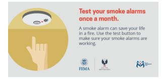
Regular Maintenance is Key: Test smoke alarms monthly by pressing the test button. If the alarm emits a weak sound or no sound at all, replace the batteries immediately. Additionally, clean smoke alarms regularly to prevent dust accumulation, which can interfere with their functionality.
