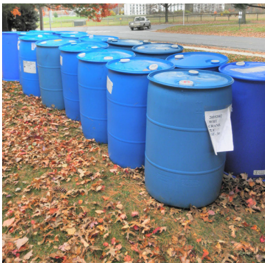
Closed top (left) and screw top (right) plastic food grade 55 gallon barrels.
