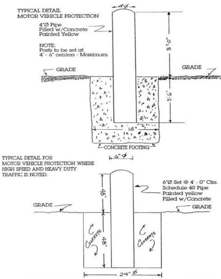
ABOVE ARE MINIMUM REQUIREMENTS FOR CRASH POSTS AT LPG INSTALLATIONS - - N.J.A.C. 12:200-3.3 (i)
